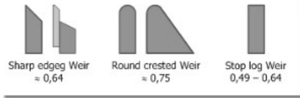
Figure 112: Examples for typical Overfall Coefficients
