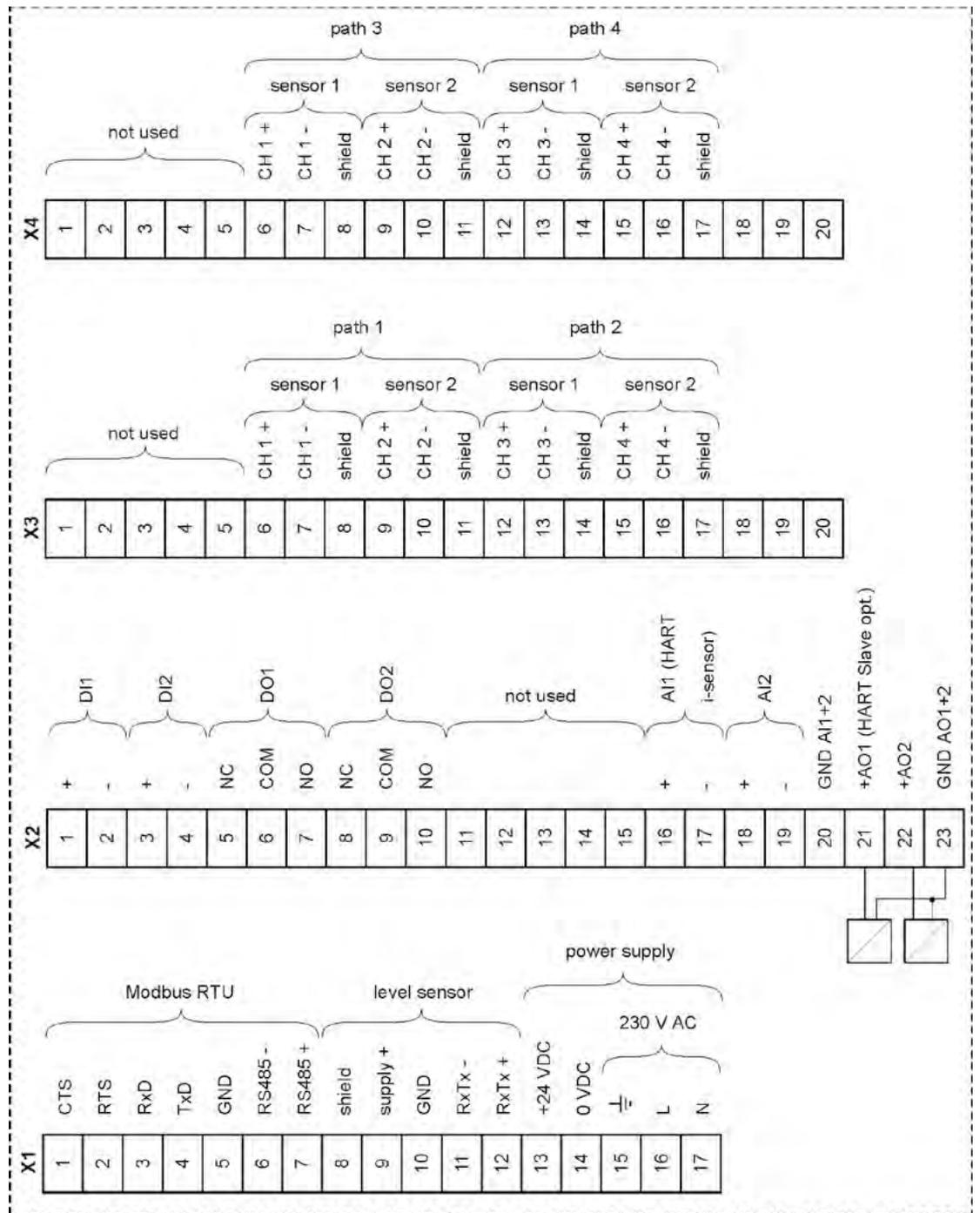
Fig. 21-4 Terminal connections NivuFlow 650 Type T4
