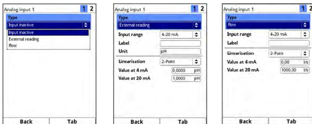
**Fig. 32-16 Analog inputs: Activation / Ext. Reading / Flow**
