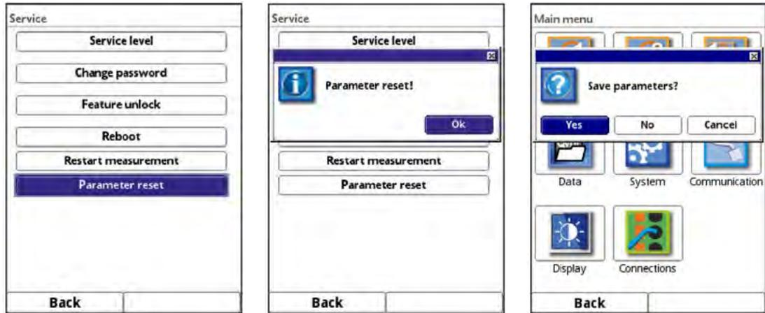
Fig. 34-12 Resetting the parameters to default settings
