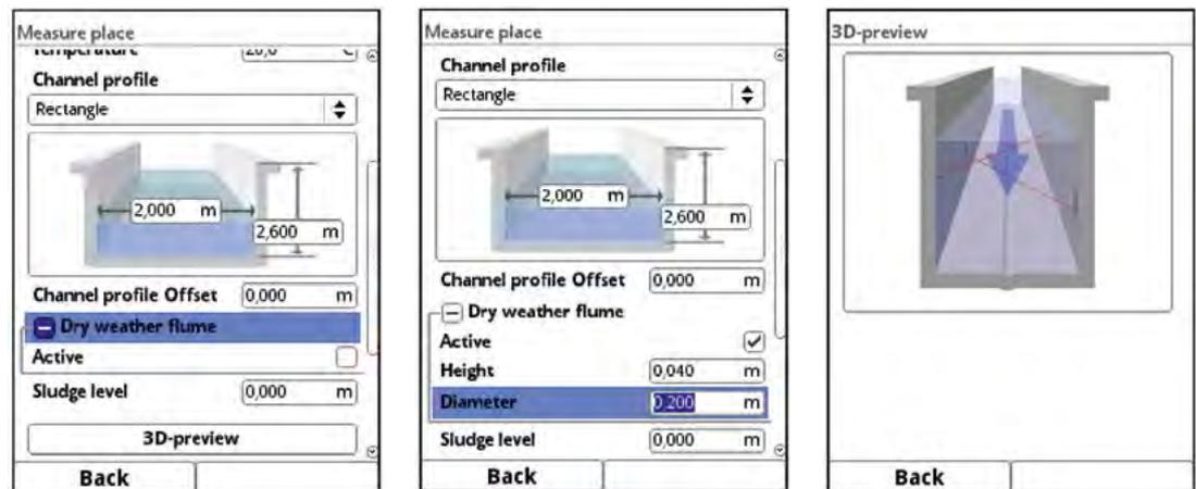
Fig. 28-8 Dry weather flume and sludge level
