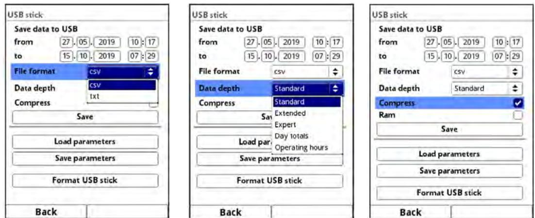
**Fig. 33-7 Transmission period / data depth / compression**
