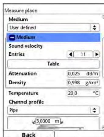
Fig. 32-3 Selecting the measurement medium
