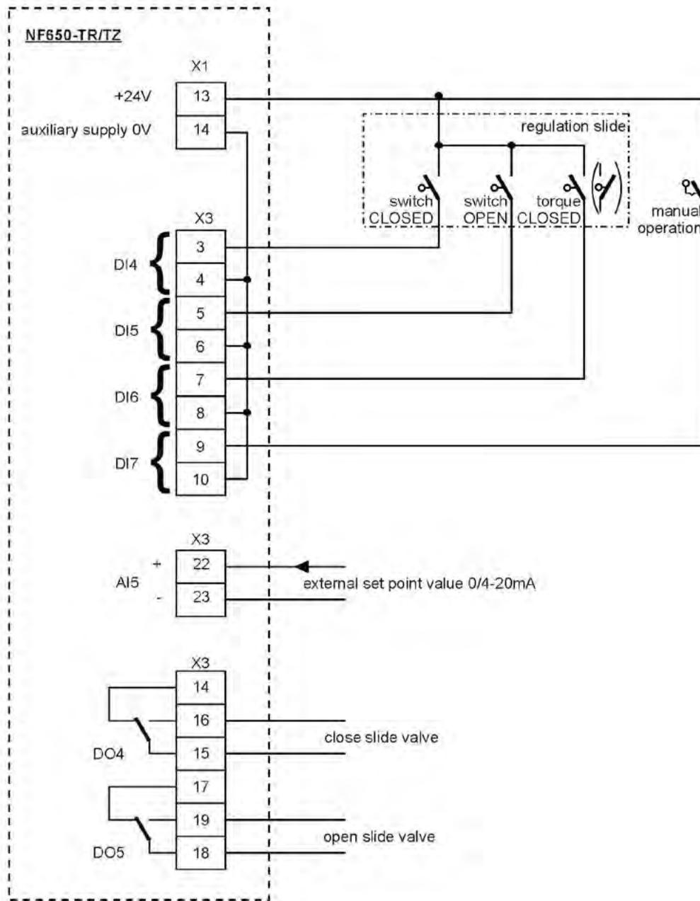
Fig. 23-2 Wiring diagram regulator mode NF650 Type TZ/TR
