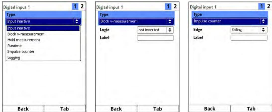
**Fig. 32-18 Digital inputs: Activation / Block v-measurement / Impulse counter**
