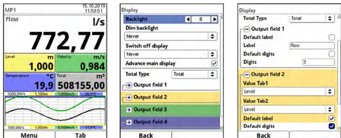
Fig. 36-3 Output fields, colours and settings
