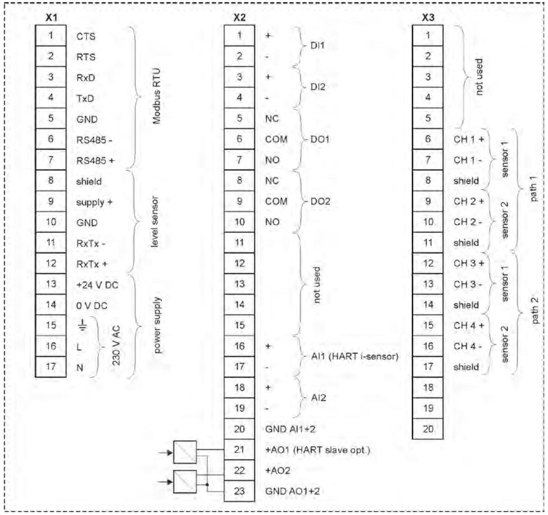
Fig. 21-2 Terminal connections NivuFlow 650 Type T2
