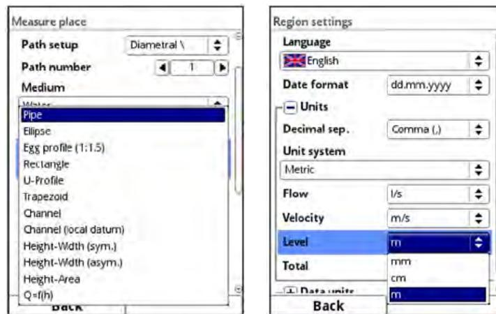
**Fig. 32-4** Selecting the channel profile / Setting the units
