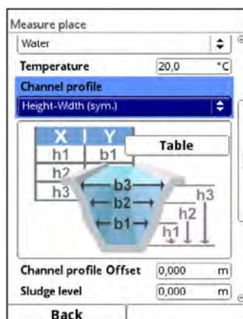
**Fig. 32-5 Setting of profile using height-width (sym.)**
