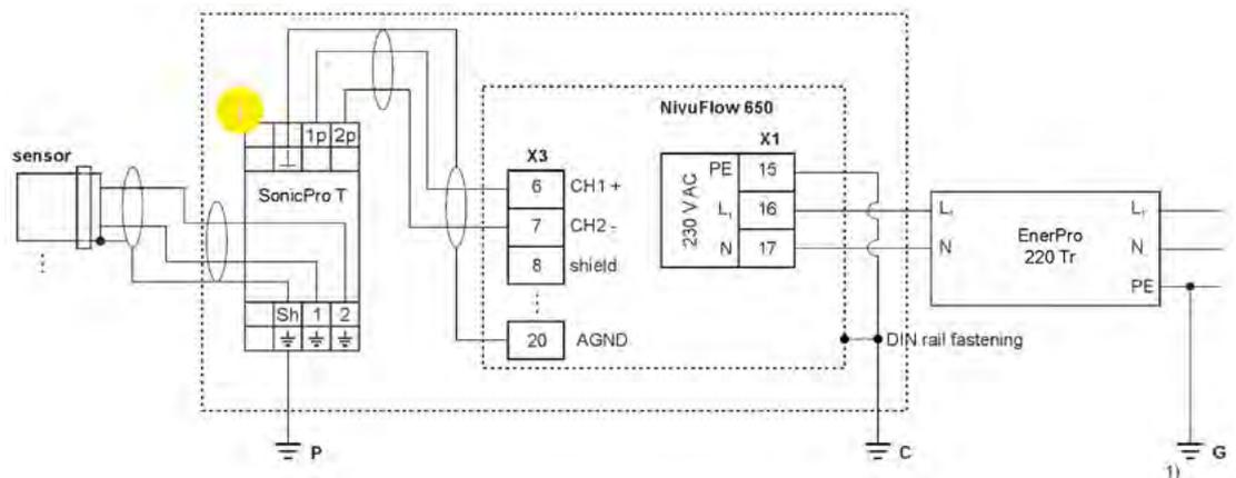
P Earth connection for the “SonicPro T” overvoltage protectors on the sensor side
