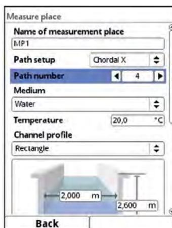
**Fig. 29-1 Select path arrangement and number of path**
