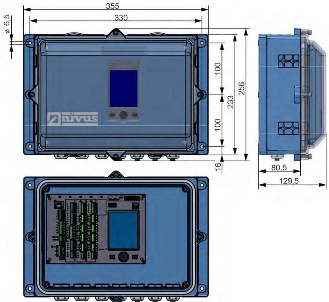
Fig. 15-3 Dimensions of field enclosure NivuFlow
