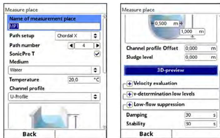
**Fig. 27-1 Setting the measurement place parameters**
