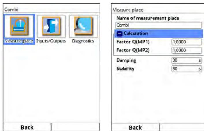
**Fig. 32-9** Setting parameters in measurement place Combi menu
