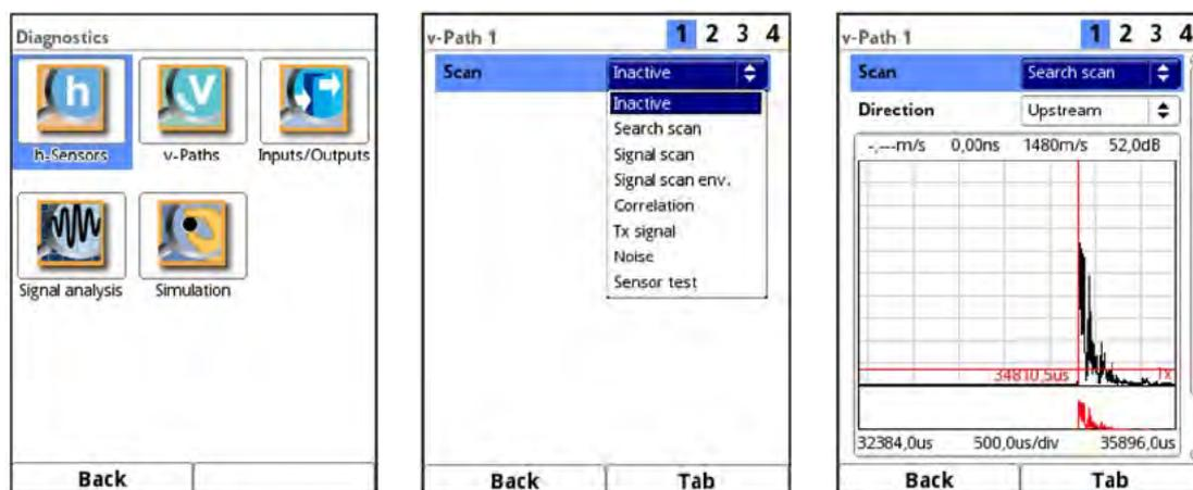
Fig. 44-1 Signal analysis Pulldown menu / search scan
