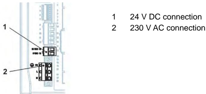
Fig. 21-7 Electrical connections of power supply NivuFlow
