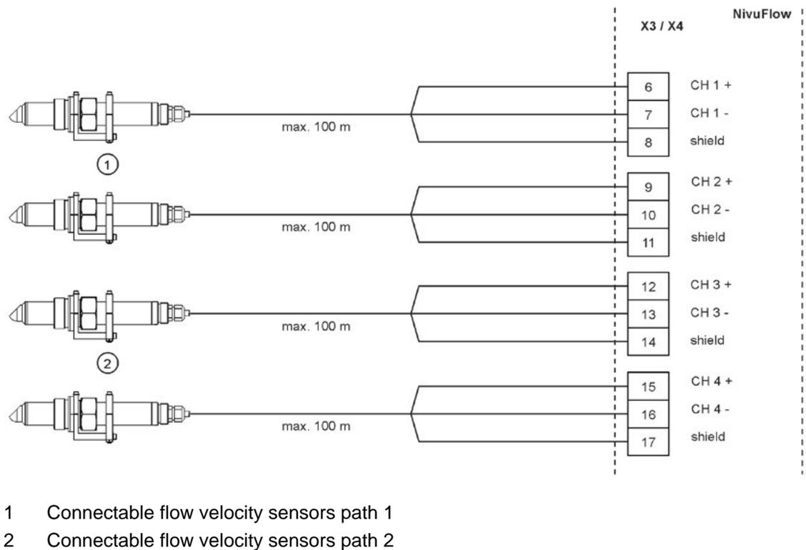
**Fig. 22-5 Connecting 2 pairs of flow velocity sensors**
