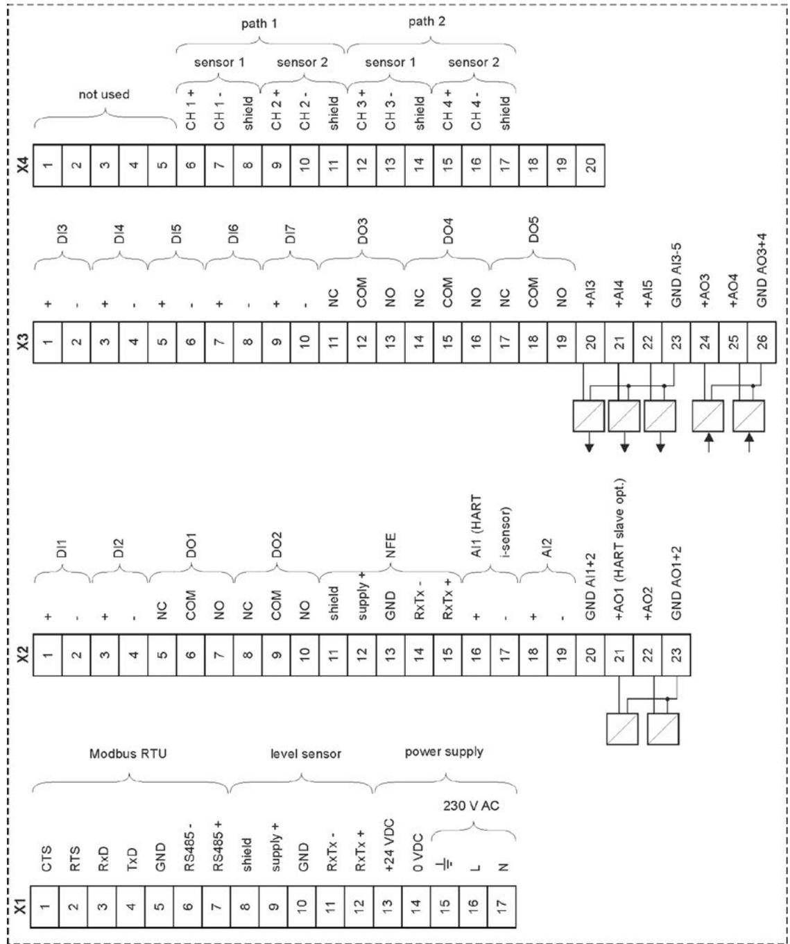
Fig. 21-6 Terminal connections NivuFlow 650 Type TZ
