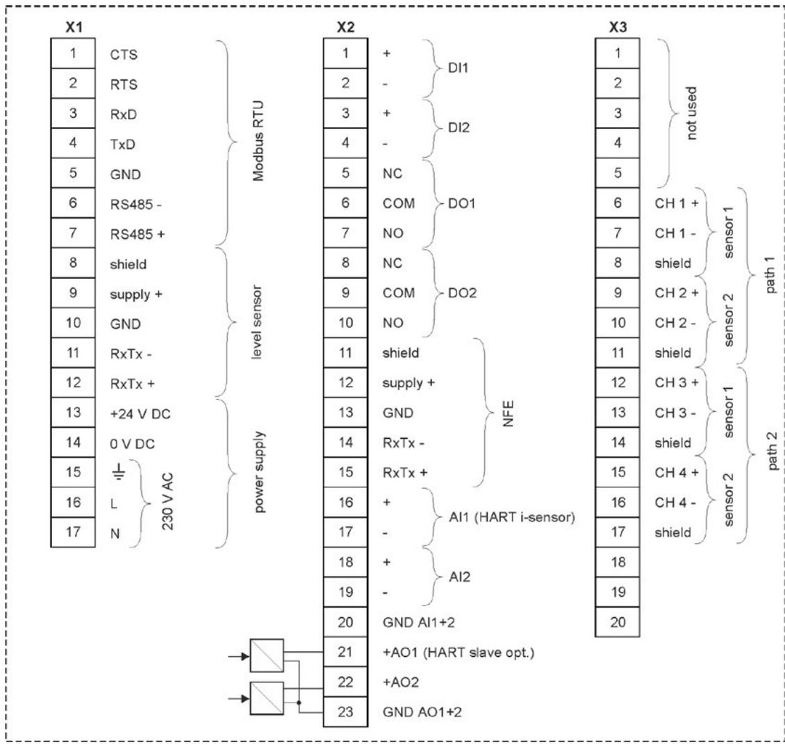
Fig. 21-3 Terminal connections NivuFlow 650 Type TM
