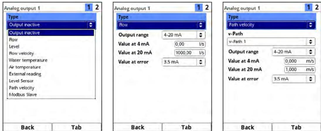
**Fig. 32-17 Analog outputs: Activation / Flow / Path velocity**
