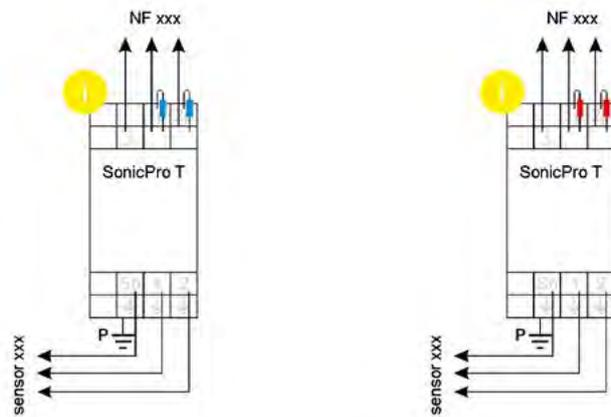
**i** Do not reverse protected (p) and unprotected sides of overvoltage protection
