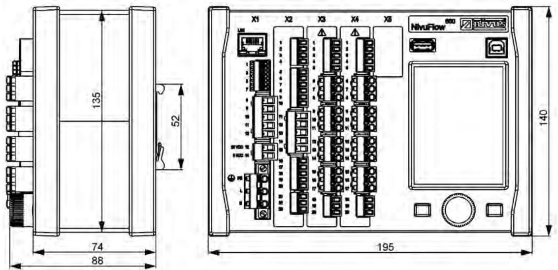
Fig. 15-2 Dimensions of NivuFlow 650 enclosure type E0
