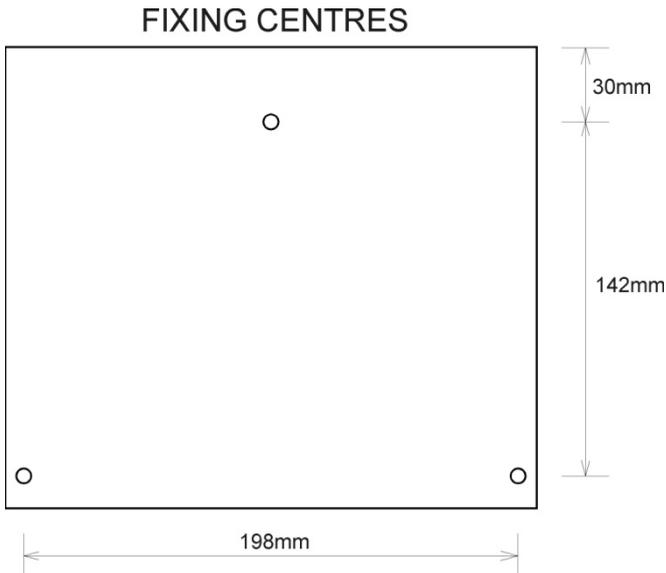
*NivuScope 2* should be mounted by drilling three holes suitable for size 8 screws (length to suit your application) and fixing the top screw in place. Hang the unit on this and fix the two remaining screws by removing the terminal access cover to access the pre drilled holes.
