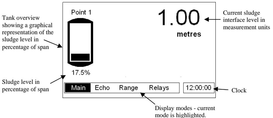
Error messages, such as “Wiper Fault”, “Status = LOE” or “Status = Failed” will be displayed on this screen, relating to the point of measure currently being viewed, when a fault condition occurs.
