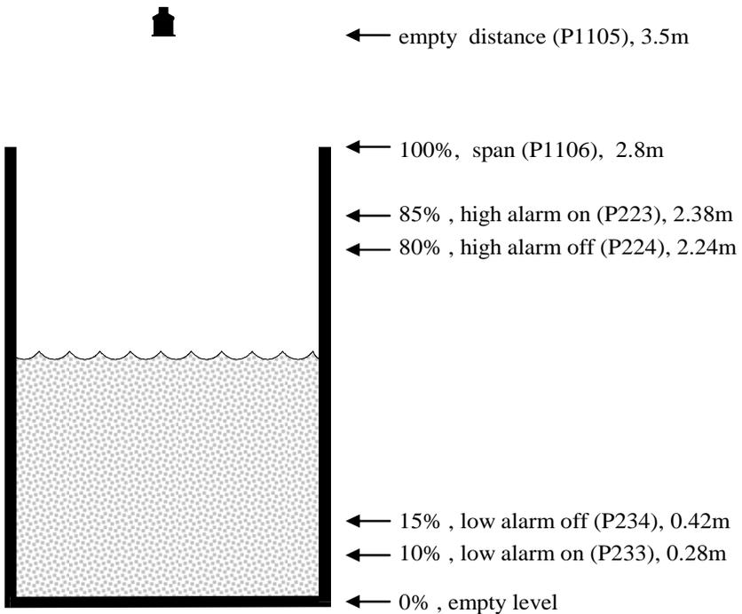
In this example, when the level rises to 2.38 m, relay 2 will come on until the level drops to 2.24 m when it will turn off. If the level drops to 0.28 m, then relay 3 will come on until it rises 0.42 m when it will turn off.
