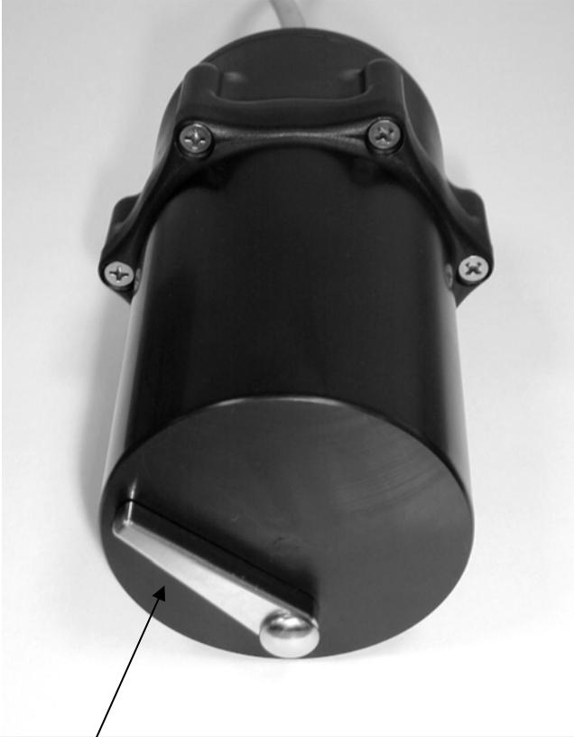
**THE ONE YEAR SENSOR WARRANTY IS VOID IF THE WIPER BLADE IS ROTATED BY HAND. THIS IS DETRIMENTAL TO THE MOTOR GEAR DRIVE AND WILL DAMAGE THE UNIT.**
